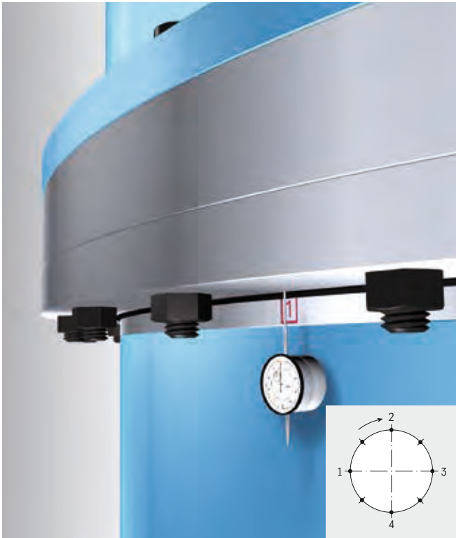
Figure 34: Basic setup for measuring the tilting clearance
